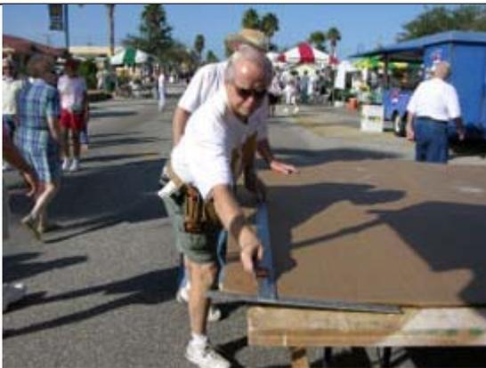
The fold (center) of the cardboard will be the bottom edge for one side of the boat. Now you must decide how wide you want the boat to be. It should be a minimum of 24" wide up to a max of 31" wide. The sides can be anywhere from 8" to 10" high, but we have found from experience that 10" works very well.
