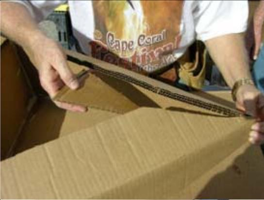
While holding the bow together, cut through the two 4" top rails so you have a clean cut and they will fit together. Cut a scrap piece of cardboard to fit underneath them. Use contact cement to glue the front and the scrap under the cut you just made. You can use screws to temporarily hold them together.
