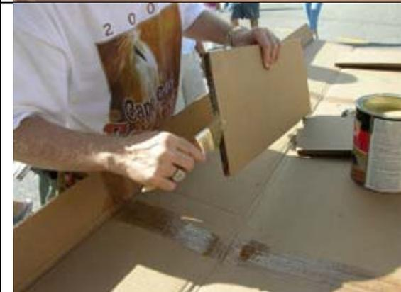
Use an inexpensive paint brush to apply the contact cement. You also need to apply contact cement to the bottom and side edges of each piece and to the bottom and sides of the boat where the braces will be installed. In the picture above you can see where we marked along the edge of the center bulkhead so we know where to brush on the contact cement.
