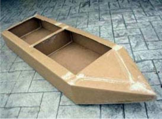
Cut two more piece of cardboard 2" wide to glue to the tops of the middle and rear bulkheads. These may also be held in place temporarily with wallboard screws.
