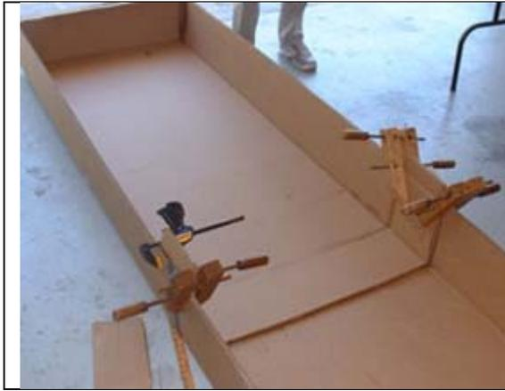
If you want a longer boat, pick up two sheets of cardboard from Lowes. Bend the second sheet to match the first sheet. Butt them together and splice them as show using contact cement.
