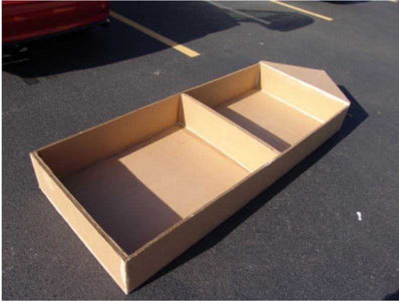
This is the completed boat, with a 33" width, ready to have the open ends filled or taped and then painted.
