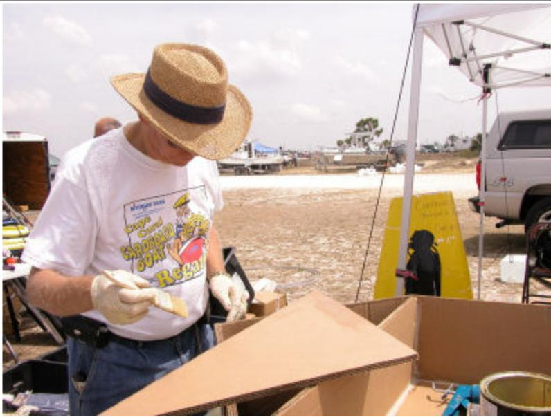
Again, apply contact cement to all the joining surfaces and once the cement is dry to the touch, place them together. You can use duct tape to hold the pieces together.
