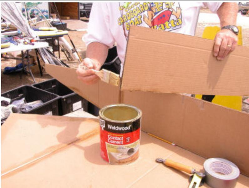
Apply contact cement to all the surfaces to be joined, including the front bulkhead.
