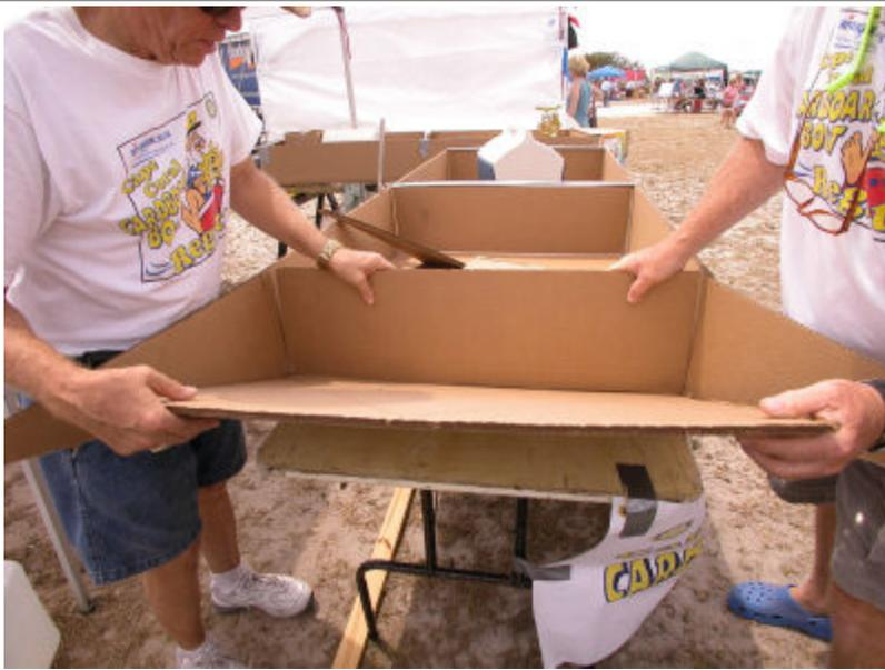
Place your front bulkhead in and use the screen roller to score the cardboard where it will be bent to create the slope of the nose.
