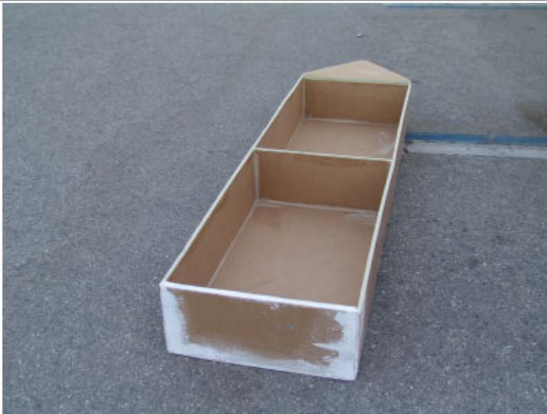
This is a boat built with a 24" width. Notice we used patching plaster to smooth out the edges after we filled them with construction adhesive. Normally it is better to use the patching plaster after you have applied the first coat of paint sealer.
