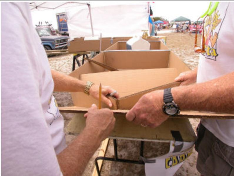
Hold the the two sides together so they meet at the center line you marked earlier. Hold the pieces together as you mark the bottom piece along the outside walls.
