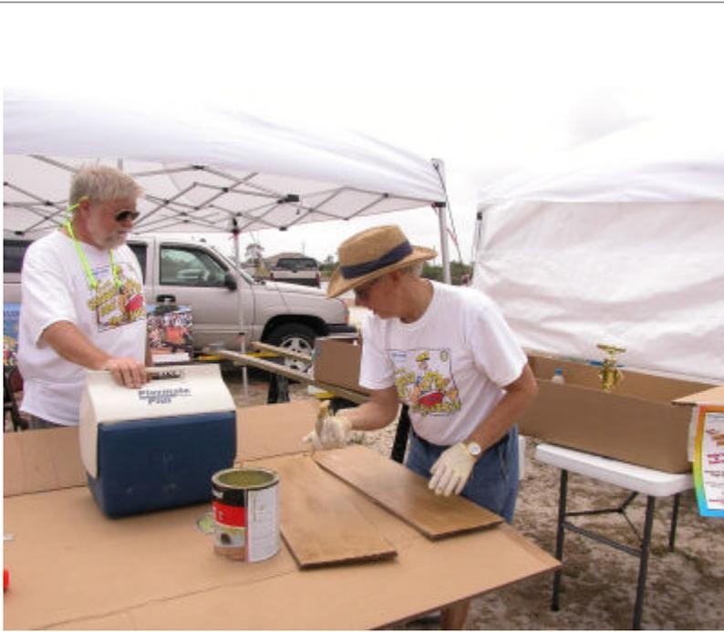
Use an inexpensive paint brush to apply the contact cement to the sides of the two pieces that will be installed in the rear for the transom. You also need to apply contact cement to the bottom and side edges of each piece and to the bottom and sides of the boat where the braces will be installed.
