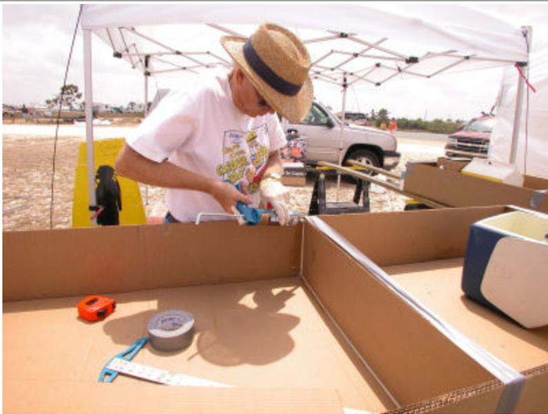
Once the braces are in, you can apply a bead of construction adhesive along the sides and the bottom of each piece. This provides additional strength and it seals the pieces from water.
