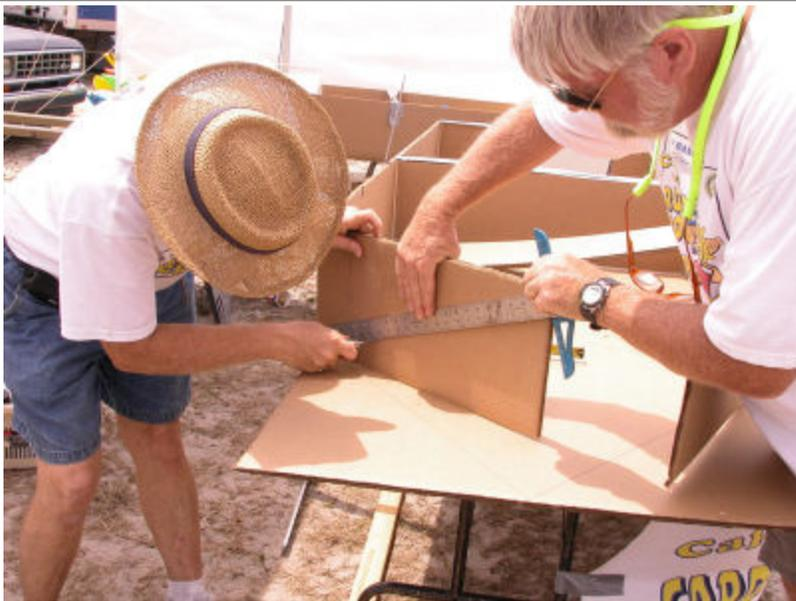
Using a straight edge, mark a line on both sides where you want to cut. The line will go from the front down to the bottom where your bend meets the bottom of the boat.
